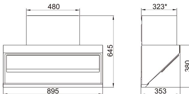
The marked sizes are for reference only, the depth dimension includes machine feet. (Unit: mm)
