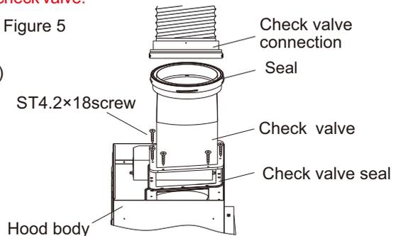
Note: During installation, straighten the aluminum exhaust pipe to avoid noises in semi-stretched state. Excess part may be cut with a wire cutter.
